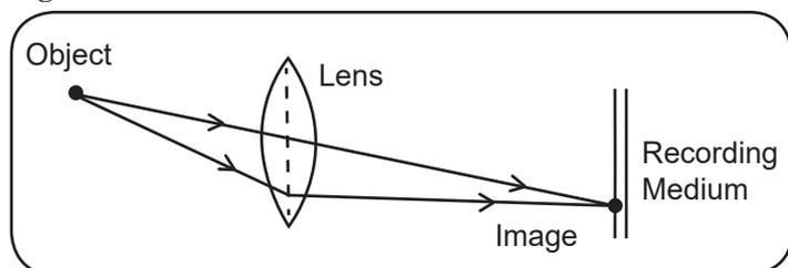
This system is basically identical for both a film camera and a digital camera. More complex systems may include mirrors or prisms as part of the focusing and control systems. A simple lens on its own would only focus objects at a fixed distance. By moving the lens back and forth, it is possible to focus objects which are at different distances.
