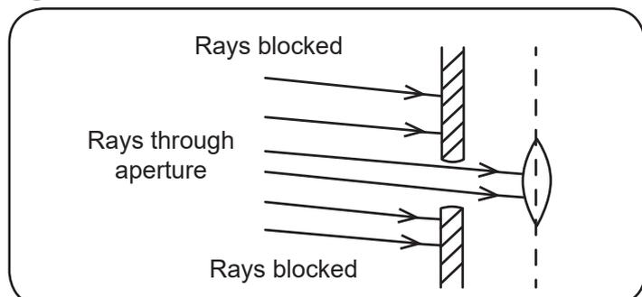
It is best to have the aperture as small as possible. This increases the *depth of focus* of the camera. Objects at slightly different distances can be focused without moving the lens. A smaller aperture also reduces the amount of aberration (distortion) of the image. This is partly due to different wavelengths of light (different colours) travelling at slightly different velocities through glass, thus refracting slightly differently.
