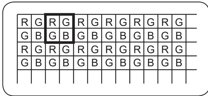
Notice that in each block there are 2 green filters, but only 1 red and 1 blue filter, causing the final image to be biased towards the green part of the spectrum: however, our eyes are more sensitive to green light than to red or blue light, so the final image is seen as more “true-to-life” by our eyes.
