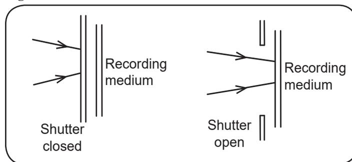
The shutter allows the incoming light rays to reach the recording medium for only a set amount of time. Obviously, the shutter and aperture work together to achieve the ideal amount of light reaching the medium.
