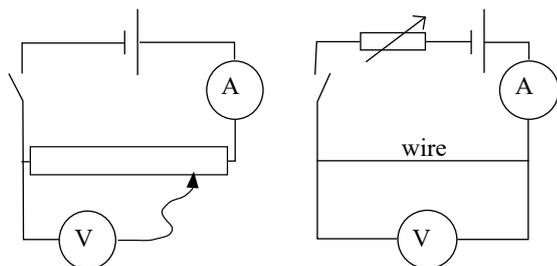
power-supply, wire, (variable resistor) and ammeter in series with voltmeter connected across wire
