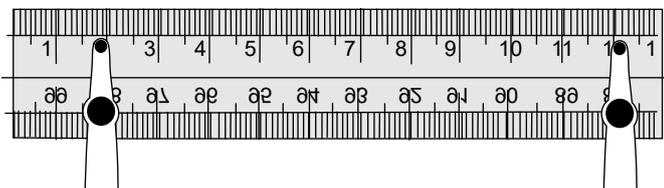
(c) With the outer-edges of the croc-clips aligned to the ruler markings
