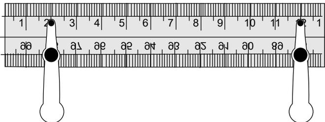
(b) With the inner-edges of the croc-clips aligned to the ruler markings
