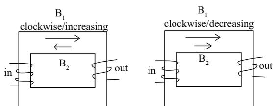
At both instants shown, the applied magnetic field,  $B_1$ , is in the clockwise direction. However, in the first diagram, it is increasing; in the second diagram, it is decreasing. In each case the induced magnetic field,  $B_2$ , will be in a direction to oppose the change in the applied field.
