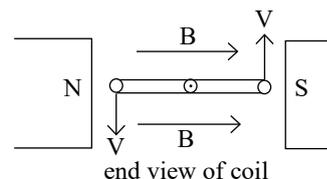
And, as before, Lenz tells us that this induced current will effectively work against the applied current, reducing the speed of the motor.
