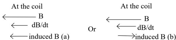
In (a), the induced magnetic field will cause the magnetic field at the coil to increase faster. This increases the induced current. The electrical energy dissipated in the circuit becomes greater and greater, but there is no source for this increased electrical energy. The Law of Conservation of Energy is violated. So, the induced field cannot add to the increasing magnetic field from the bar magnet.
