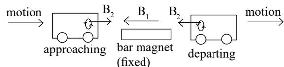
The diagram shows how the magnetic fields repel each other as the carriage approaches and attract each other as the carriage departs. This will result in a braking effect throughout the whole of this motion.
