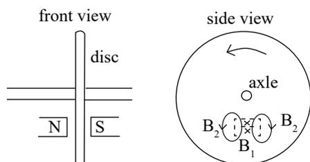
On the portion of the disc approaching the magnet, the induced magnetic fields will oppose the applied magnetic field; on the portion leaving the magnet, the induced magnetic fields will support the applied field. At both edges, the effect will be to slow down the rotation of the disc (and the speed of the vehicle). Again, in energy terms, some of the kinetic energy of the vehicle is turned into Joule heating in the disc.
