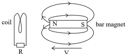
As the magnet approaches the coil, the magnetic field (due to the bar magnet) in the vicinity of the coil will be as shown below, and will be increasing in magnitude.
