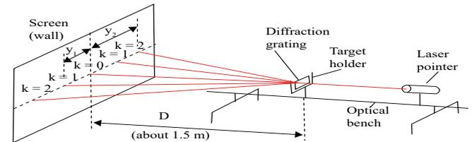
The diagram shows a simple set-up to find the wavelength of laser light using a diffraction grating.
