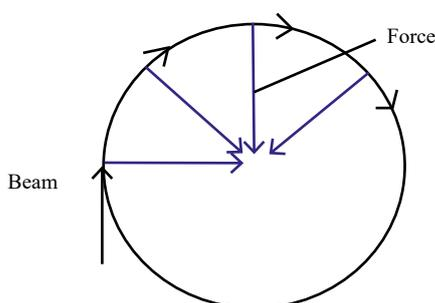
An electron beam forced into circular path by uniform magnetic field applied into page is shown above.
