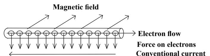
This then corresponds to a conventional current going from right to left. As the force on the wire is downwards, this force can be measured by mounting the wire on a top pan balance.
