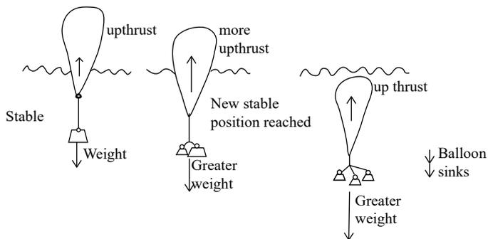
In the first case, if the float sinks further the buoyancy force (or “upthrust”) will increase.
