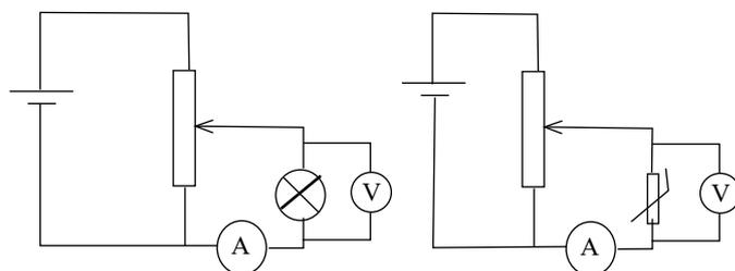
The circuit on the left is often used to measure the voltage-current characteristics of a light bulb. We can adjust the rheostat to change the potential difference across the light bulb, and record the readings on the voltmeter and the ammeter, which we then use to plot a graph of V against I.
