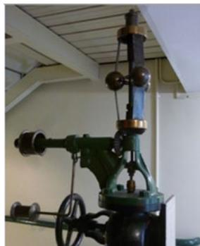
The heavy balls are attached by springy metal to the central shaft. The faster the engine goes, the more rapidly the shaft spins, which flings the masses outwards.
