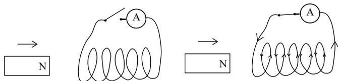
As the magnet on the left moves into the coil on the right, an e.m.f. (i.e. a voltage) is created across the terminals. If the switch is closed, the ammeter will show a reading. If the magnets were strong enough, you could light a small lamp or drive a little motor.
